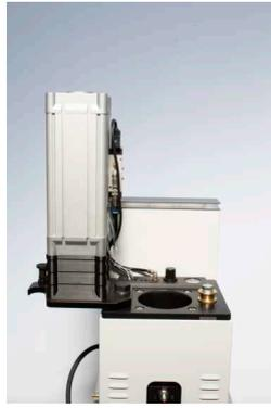
Open lid with swivelled out pressing cylinder for refill
