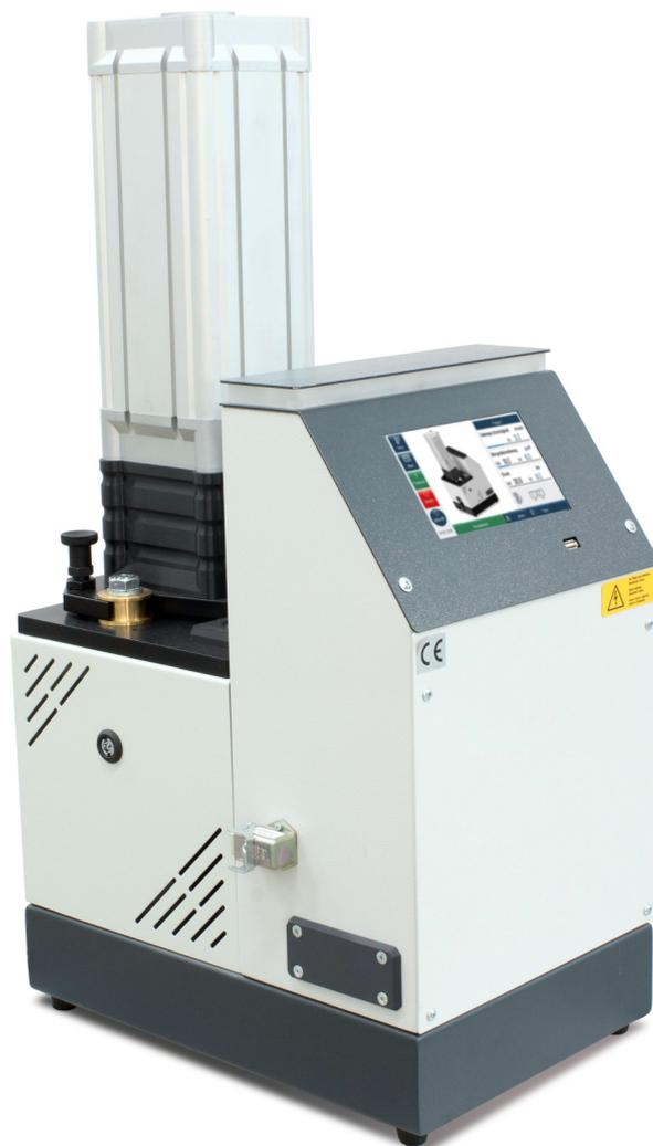
Maintenance friendly and pneumatic driven slug-melter (melting press) in bypass-free, filter- and pump-less design without dead spaces, for gentle and on-demand pre-melting, re-filling or dosing of moisture curing hotmelt adhesives in 2 kg candle packaging. Preferred use for filling roller-reservoirs for spine-gluing in bookbinding machines, edge-banding machine in furniture industries, or for feeding volumetric gear-heads in automotive applications.
