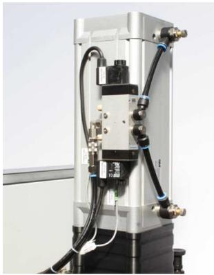
Piston position transmitter and pneumatic control valve at high volume cylinder drive
