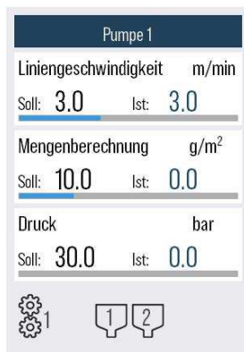
"Dosing meter" menu - automatic speed control according to quantity specification in g/m 2 or g/lfdm
