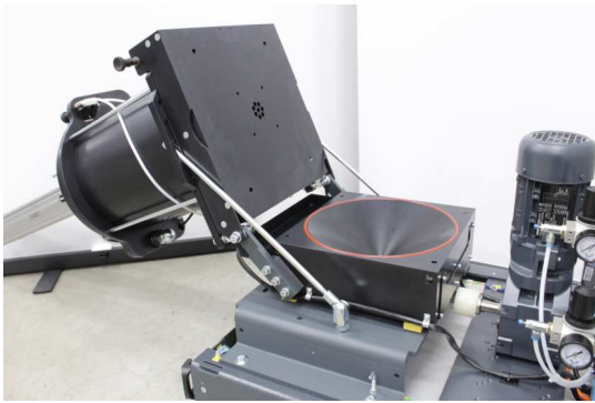
Maintenance-friendly design with hinged melting funnel
