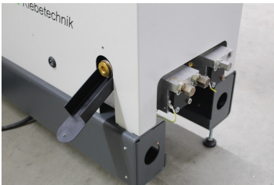
GS20 as double pump version with glue release device
