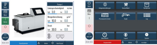
FlexControl start screen - Touch panel Operating unit
