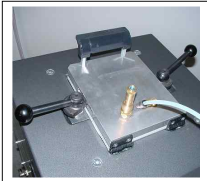
PUR-model with airproofed lid
